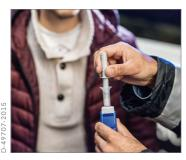
2. Insert the sampler into the funnel opening
