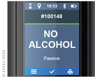
The 2.4" colour display provides information, notices and warnings
